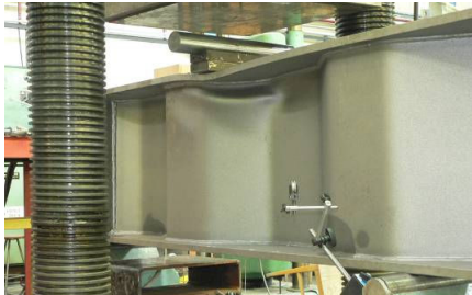
Figure 51: Experimental and numerical failure modes - specimen #2.
