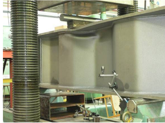
Figure 36: Failure mode of test specimen #1.
