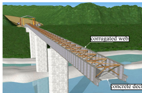
Figure 3: Incremental launching of a corrugated web bridge, from [1].
