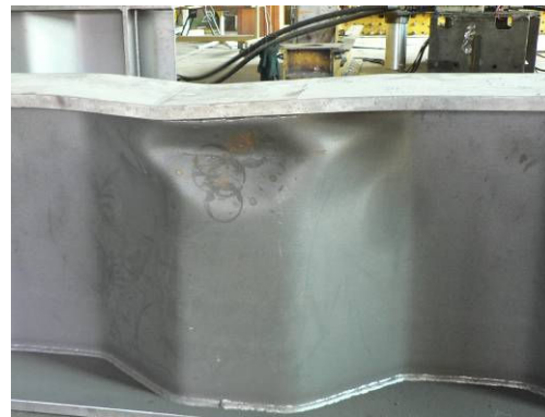
Figure 39: Failure mode of test specimen #4.
