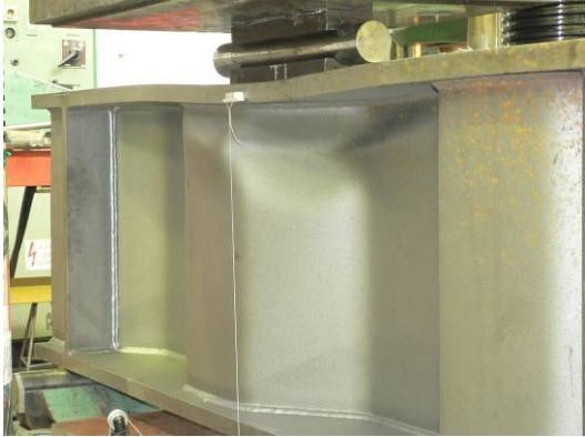
Figure 44: Failure mode of test specimen #9.
